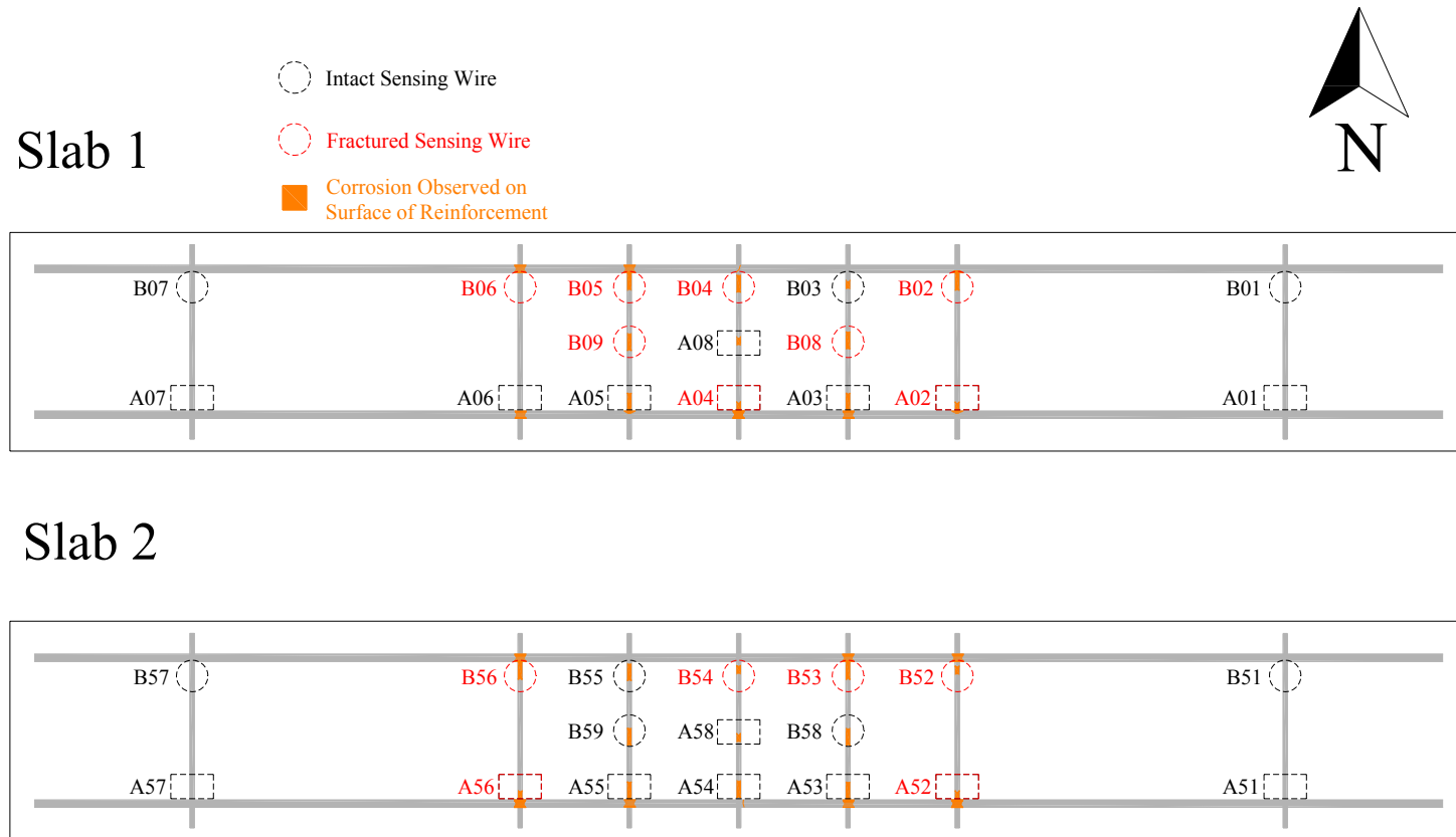
Figure 4-23 Extent of Corrosion on Reinforcement Adjacent to Sensors
