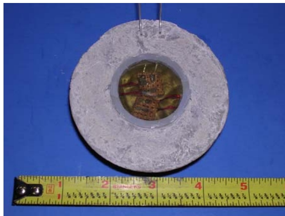
Figure E-9 Epoxy Core Visible on Top of Sensor
