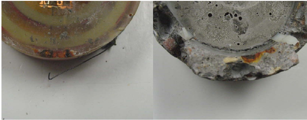
Figure 3-14 Autopsy of Prism Containing B27
