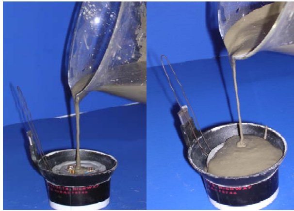
Figure E-4 Mixture Poured into Mold Containing Sensor
