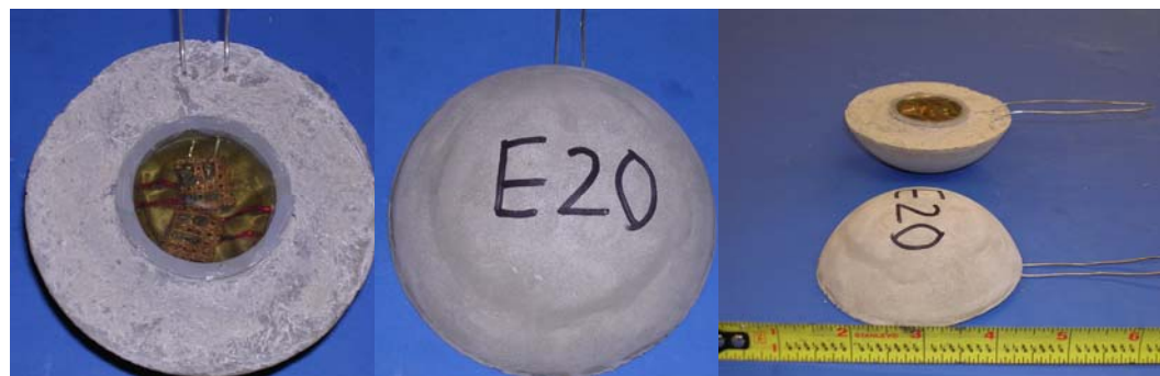
Figure 7-9 Sensor with Fiber-Reinforced Cement Paste Housing with Epoxy Core
