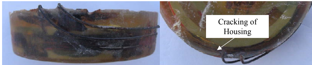
Figure 6-1 Black Corrosion in the Housing of Sensor B52
