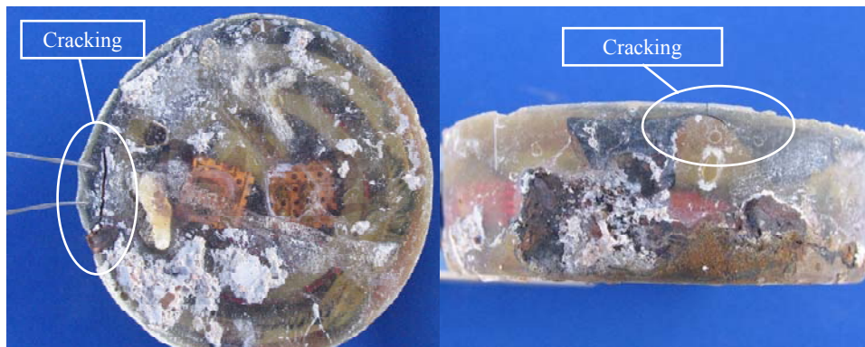
Figure 5-28 Cracking of Epoxy Housing of B152
