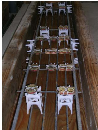
Figure 4-4 Layout of Sensors and Steel Reinforcement
