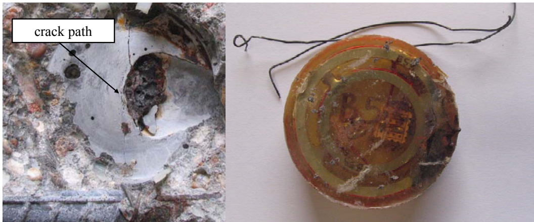
Figure 4-34 Crack Path Intersecting Sensing Wire of B53 and Reinforcement, Causing Corrosion of Both
